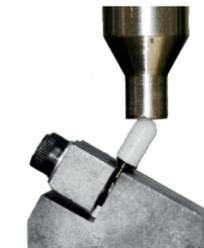
No significant difference in static fatigue strength between DESS AURUMBase® and DESS Ti Base in standard ISO 13485 test using Zirconia caps despite AURUMBase® having a 33% shorter shaft.
